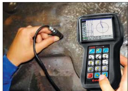
Application of special-purpose SS170K13DAO and SS340K09DAO probes in protective cases together with ALARM units and digital signal processing will allow to eliminate the influence of interfering factors such as roughness, edge effect, ECP separation from the testing object surface etc.
