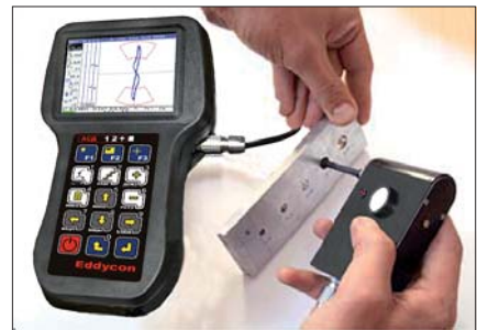
Circular scan permits an operator to locate the defect in the hole.
